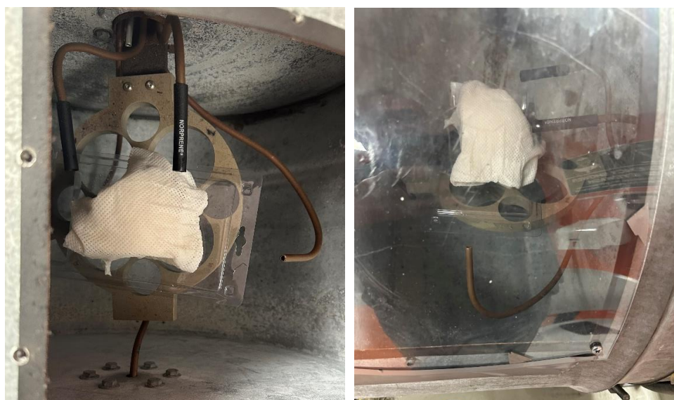
Figure 3. Location of Gelair™ AB inside rotational aerosol chamber
